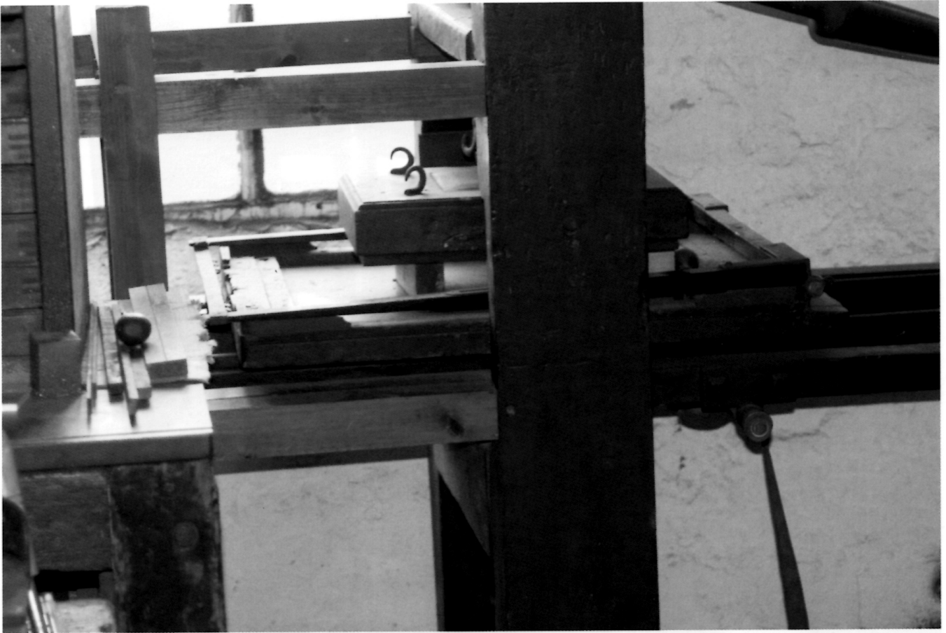
GB7. Detail of the press, showing the cheeks, platen, coffin etc.
