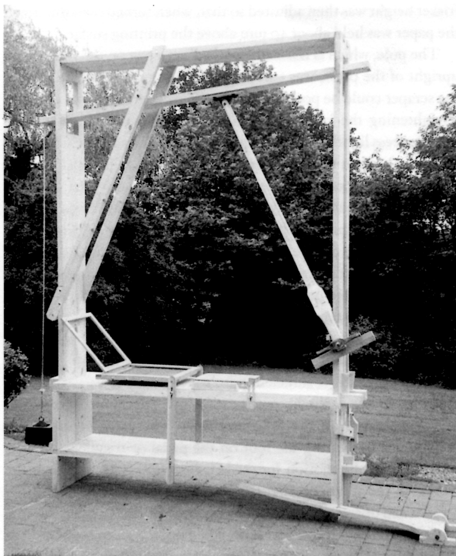
7. The reconstructed press showing the tympan and frisket lying open and the pole 'parked' on its hook.
