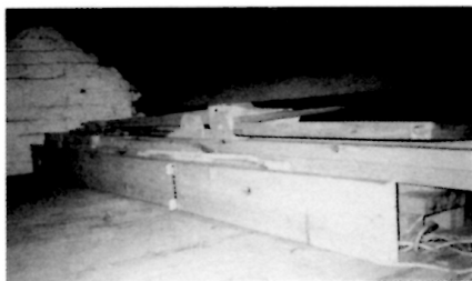
9. The press after dismantling. It occupies a space of about 3500 × 650 × 650 mm.
