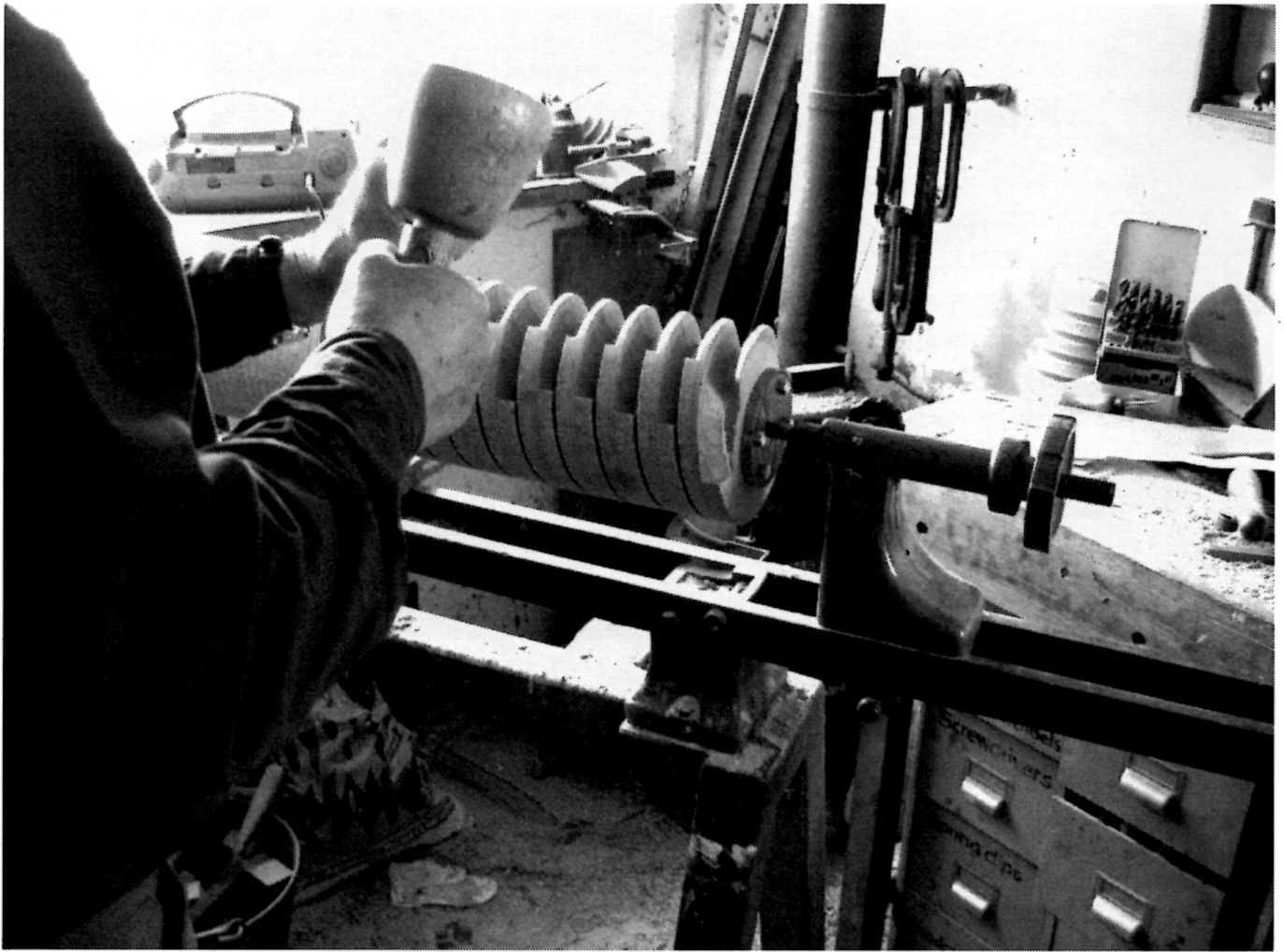
19. Cutting out the thread with mallet and chisel.
